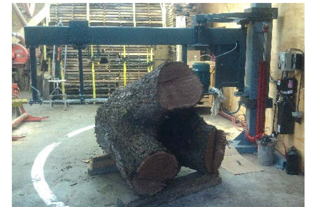
To cut logs up to 6' in diameter, Brian designed and built his own pivoting log slabber for one-sixth the price of a commercial version.
